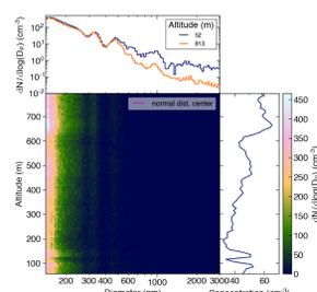
Measurements of aerosol size distribution and number concentration from the Printed Optical Particle Spectrometer (POPS) mounted on the ARM Tethered Balloon System for 26 July 2016 are shown at left. Consistent with the ground-based and aircraft data presented here, aerosol loading is enhanced at higher altitudes in a layer distinct from the surface layer.
