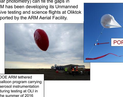
DOE ARM tethered balloon program carrying aerosol instrumentation during testing at OLI in the summer of 2016
